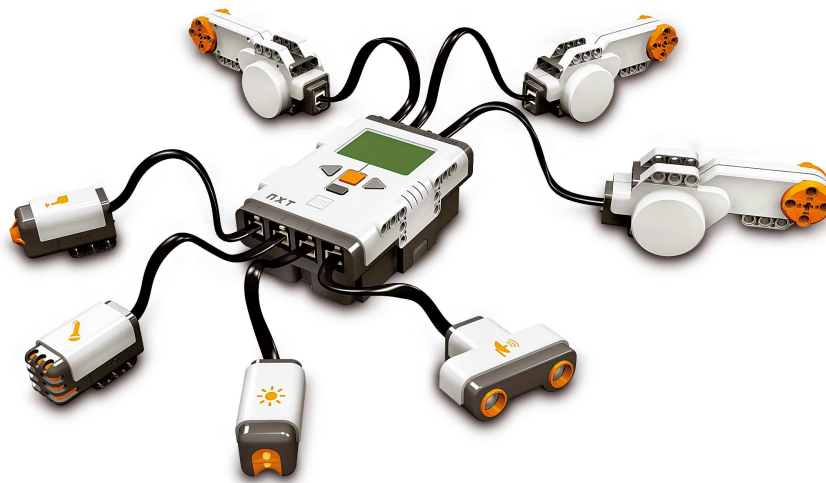
Figure 4: Lego NXT with Sensors
