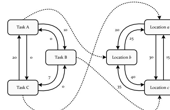
$$\mathbb{O} = t_{AB} \cdot (d_{bc} + p_{BA}) + t_{AC} \cdot (d_{ba} + p_{BA}) + t_{BC} \cdot (d_{ca} + p_{CB}) + t_{BA} \cdot (d_{cb} + p_{CB}) + t_{CA} \cdot (d_{ab} + p_{CA}) + t_{CB} \cdot (d_{ac} + p_{CA}) + c_{bA} + c_{cB} + c_{cA} = 3637$$
